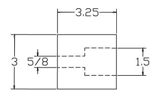
TB-10 is molded from a nylon & polyester fibre reinforced rubber of 80 (+ or -) 5 durometer, and has an average impact resistance of 95% under ASTM 1170.
