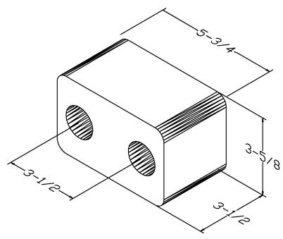
TB-20 is molded from a nylon & polyester fibre reinforced rubber of 80 (+ or -) 5 durometer, and has an average impact resistance of 95% under ASTM 1170.
