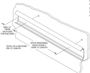
**2.** Drill holes in centerline of retainer using 1/4" [6mm] drill bit. Position retainer on wall allowing for end caps/corners. Level and mark holes. See Figure 2.
