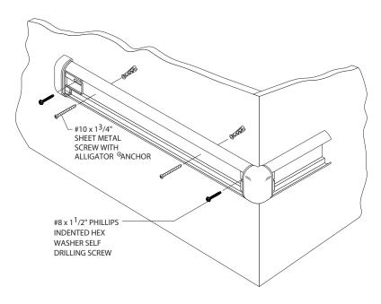
**3.** Drill marked holes on wall using a 1/4" [6mm] drill bit and position Alligator anchors into holes. Mount retainer on wall and tighten screws to secure. Slide end caps and corners onto the retainer and secure, leaving a
