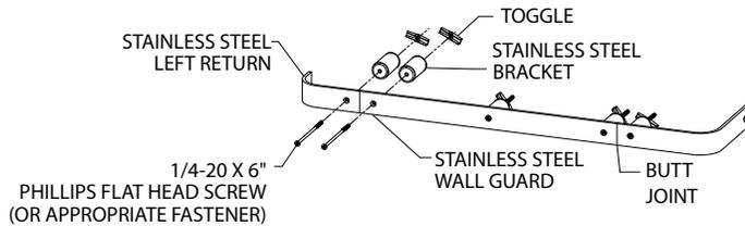
4. Loosely attach the mounting brackets and appropriate fasteners at each mounting location. When the installation involves longer lengths or is a continuous installation with corners, a single bracket is used at each side of the butt joint. See Figure 3.
