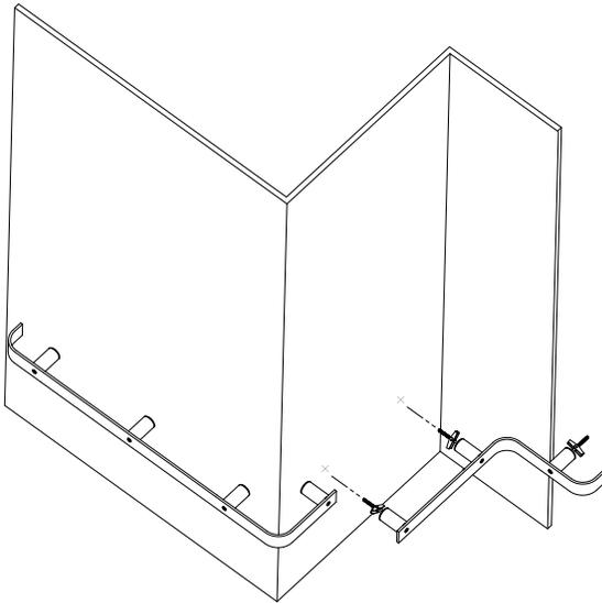
5. Starting at one end, lift the wall guard assembly to the wall, level and tighten until secure. Continue this process sequentially making sure all butt joints are aligned and tight. See Figure 4.
