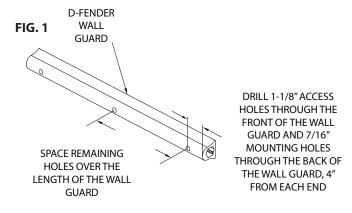
Note: Wall guards are rough-cut; cut square if needed. Height of the Wall Guard may vary over the length of the product. Match ends with similar height for best fit. To clean rubber products use water or, "Back to Black" tire cleaner for stubborn marks.
