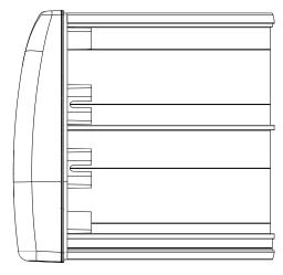
Attach End Caps and Corners to retainer, leaving 1/16" gap between Return/Corner and retainer allowing for adjustment. See Fig. 3.
