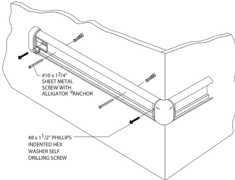
3. Drill marked holes on wall using a 1/4" [6mm] drill bit and position Alligator anchors into holes. Mount retainer on wall and tighten screws to secure. Slide end caps and corners onto the retainer and secure, leaving a
