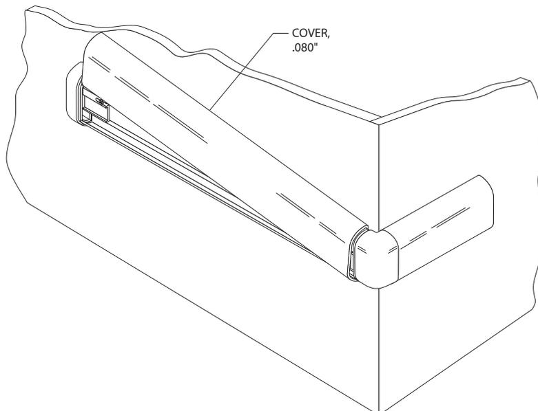
4. Cut the cover to length between end caps and/or corners. (Note: Trim factory edges square before installation). Position cover on retainer and adjust end caps and/or corners for a tight fit. Starting at one end, push cover onto retainer until it snaps into place. See Figure 4.
