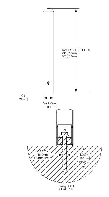
FlexCore Post 3 Post Part Numbers Height Stainless Finish 24" [610mm] CSFP-3-24 32" [813mm] CSFP-3-32 0 3/4 x 5" Redhead Tapcon Anchor LDT-3454 Washer CSFP-3-WASHER Ring CSFP-3-RING Cup CSFP-3-CUP 3/8-16 x 3" Flat Socket Head Cap Screw SCALE:1:8
