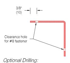
• Standard spacing: 3" (76) from each end and spaced evenly not to exceed 36" (914) oc
