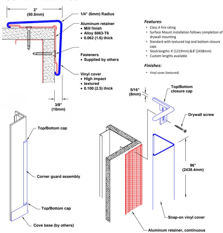
Partial height installation with top and bottom caps shown. Full height installations may not require top or bottom cap.
