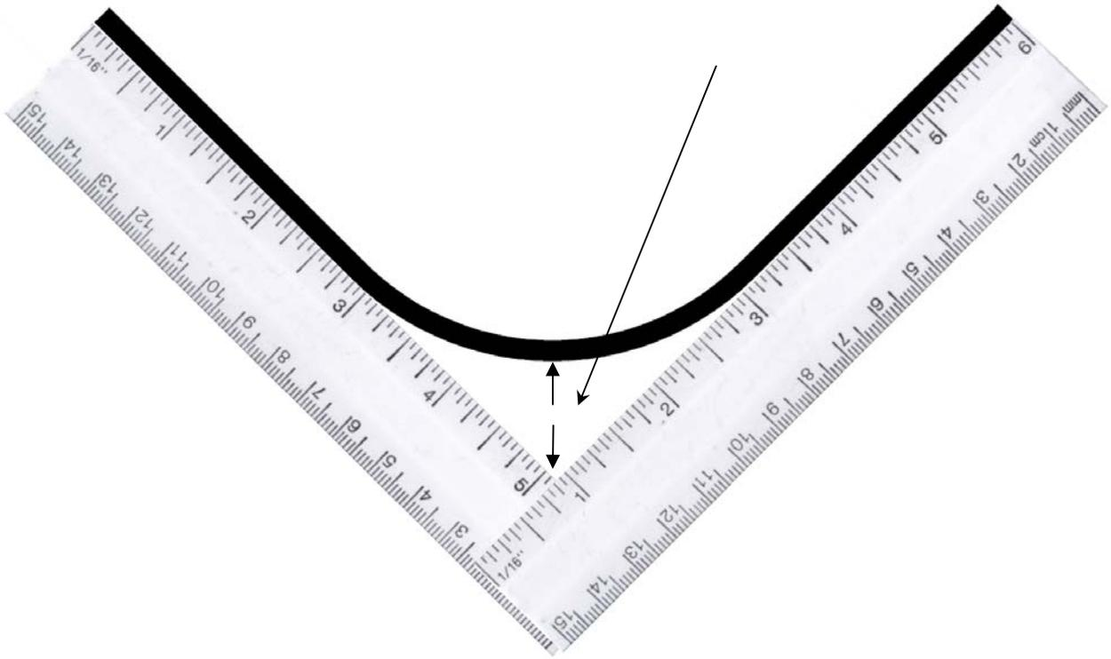
Take 2 straight edges (rulers) and lay them flush against each of the walls. Where they cross, measure straight back to the middle of the rounded corner. This measurement is the radius of the corner.
